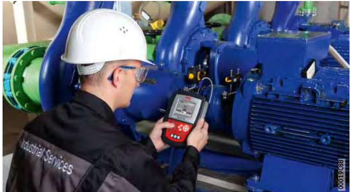
Figure 8 Shaft alignment device FAG Top-Laser EQUILIGN
